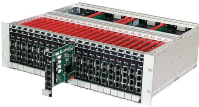
The Cubro FlexTAP 10/100/1000 allows the uninterrupted passage of full duplex data over standard Category 5/6 copper network cable. Featuring auto negotiating between 10Mbps, 100 Mbps and 1000 Mbps, this TAP duplicates the network signals, including any existing physical errors, to the transmit-only monitoring ports.
